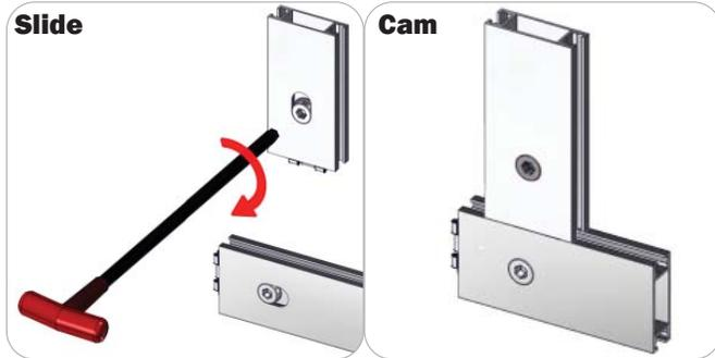
A cam lock equipped extrusion can lock to any cam lock channel. With the cam lock unlocked, set the teeth of the cam lock into the desired position on the cam lock channel. Using your allen key tool, carefully turn the lock clockwise to lock in place. Be sure to lock securely, but do not over tighten.
