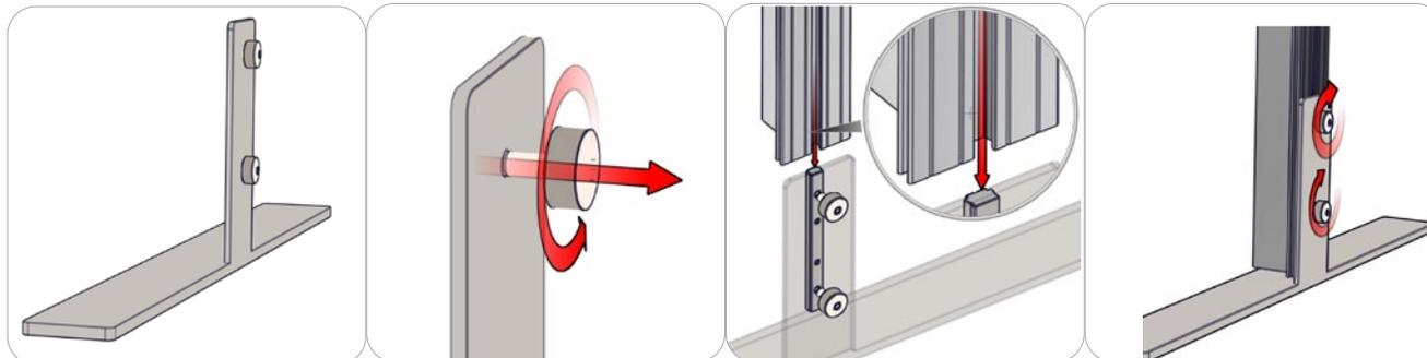
An SW-FOOT assembly consists of two thumb screws, an LN100, and SW-FOOT baseplate. Start by loosening the thumb screws (it is best not to completely remove the screws). Slide the extrusion onto the LN100 by utilizing its back cam channel. When the extrusion rests on baseplate or ground (depending on application), tighten the thumb screws to lock in place. Do not overtighten.
