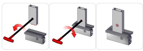
First, with the cam lock disengaged, place the cam lock teeth into the extrusion channel. Second, use the allen key tool to lock it in place. Make half turns clock-wise to engage the cam lock. Do not over tighten the lock buttons.
