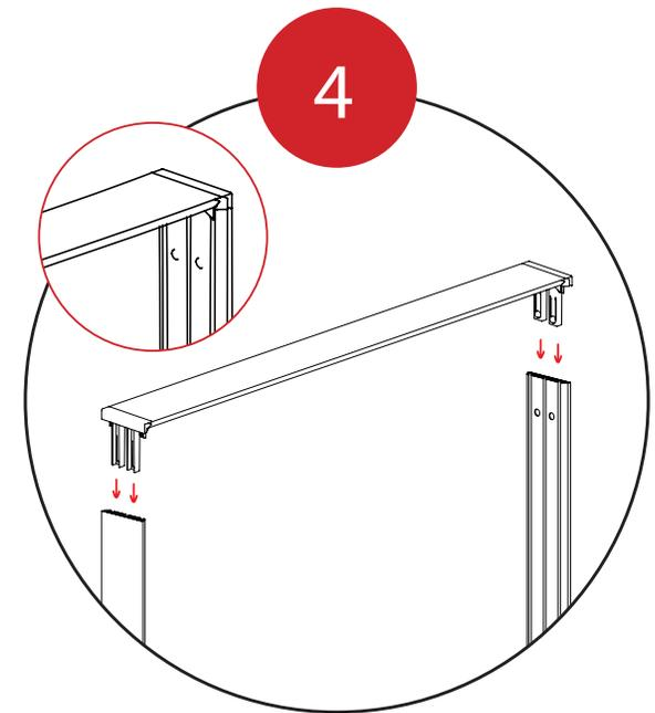
Fit the Channel Bar
