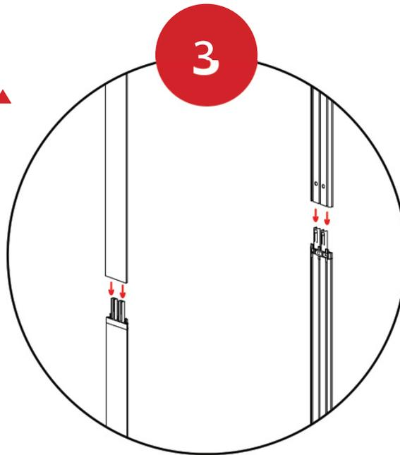
Fit the Top Extrusion ● onto the Side Extrusion Top ▲ connectors.
