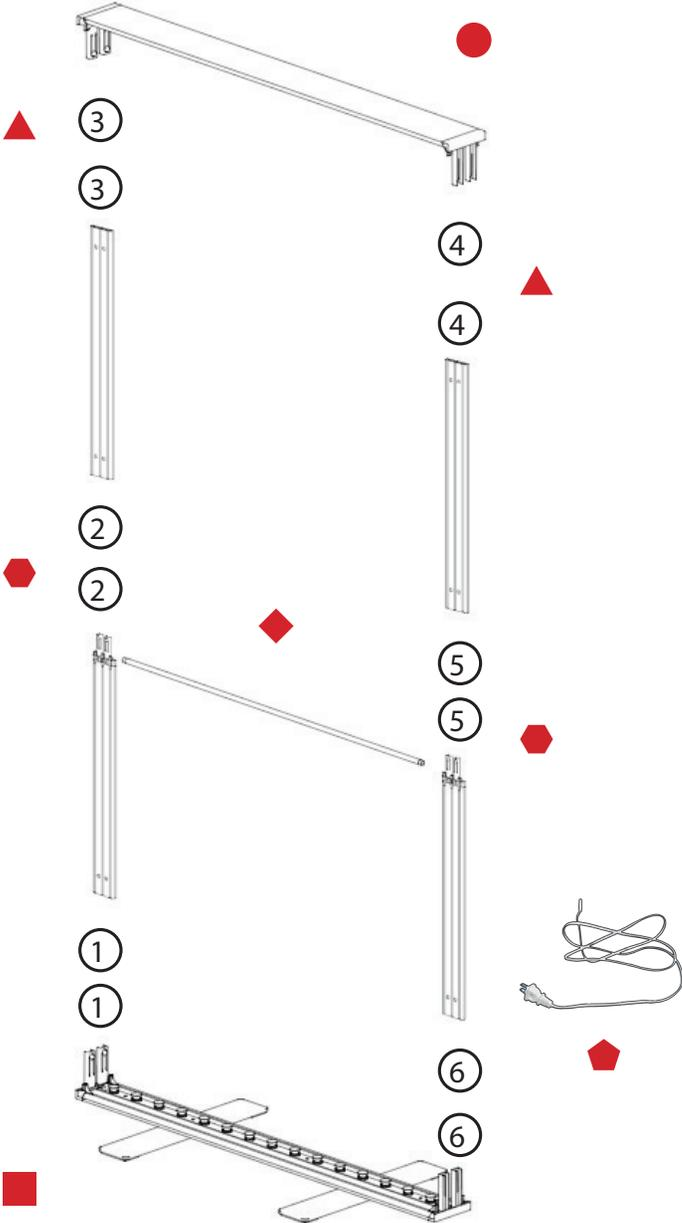
Swivel the feet of the Bottom Extrusion. ■
