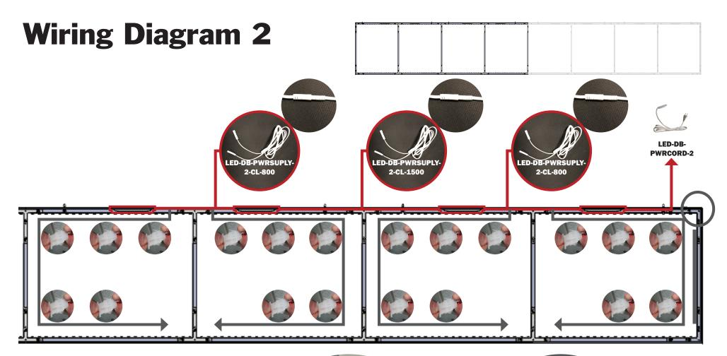
Connect the light strips along the top and bottom of the frame together with their clips per the diagram above. (right side of the frame)
