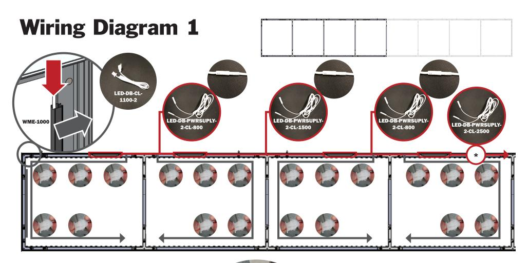
Connect the light strips along the top and bottom of the frame together with their clips per the diagram above. (left side of the frame)
