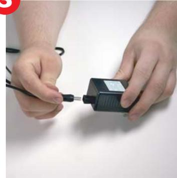
Transformer should already be attached, if not simply plug cord into transformer (make sure transformer is not plugged in).
