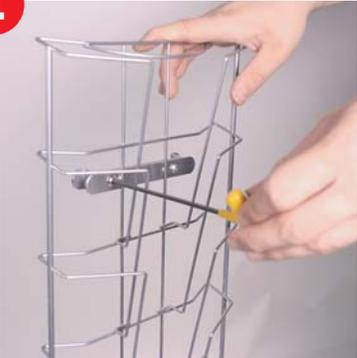
Loosen 1 screw holding the top back plate in place. Remove the other screw from the unit and let back plate hang down. Take same steps for the bottom back plate.
