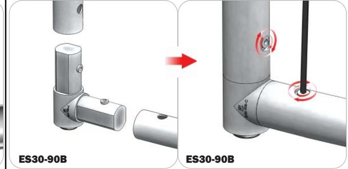
Compress one unlocked end of the connector and slide it through one tube end. Compress the other end of the connector and slide the second tube on. Lock both screws carefully using your allen key tool. Be sure to lock securely, but do not overtighten.
