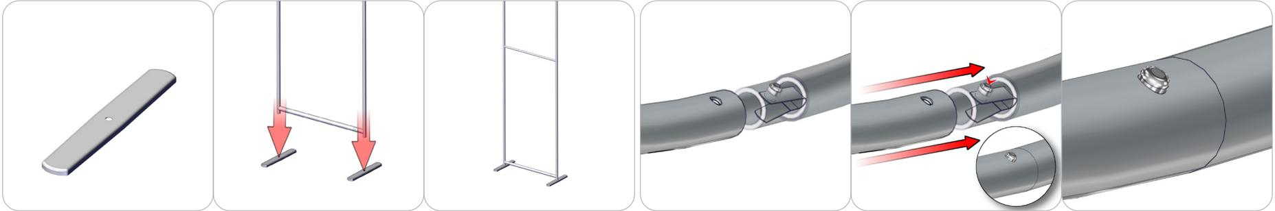
First, attach the base plate with the M10 screw. Once the base plate is in the desired position, fasten the set screw to hold the insert in place.
