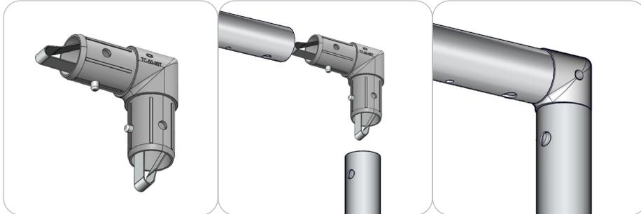
Take the plastic connector and make sure the snap buttons are in proper position for the frame tube holes. Simply press the snap button with your thumb and carefully slide the tube onto the connector. The snap button should pop through. Some twisting may be necessary to assure the snap button has popped all the way through the tube hole. Do not force the connection and be careful with the tube edges, they may be sharp.
