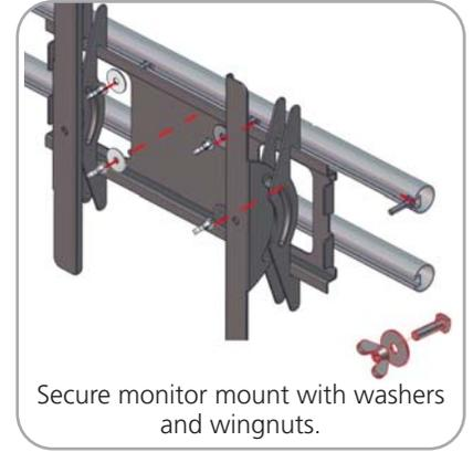
Secure monitor mount with washers and wingnuts.
