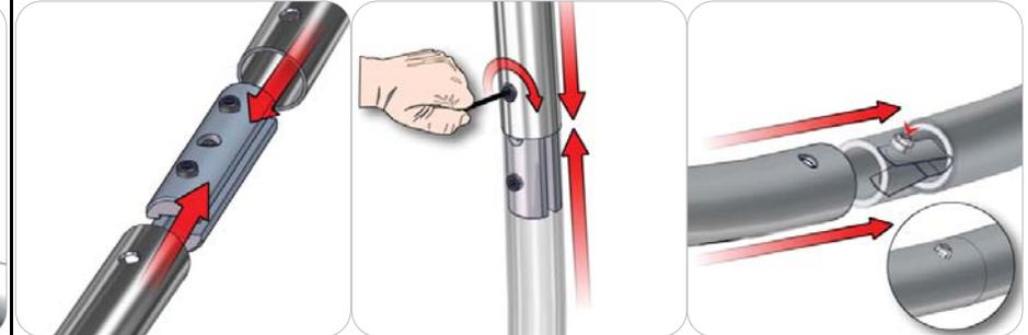
Compress the unlocked connector and slide one tube onto each end. Lock both screws carefully using your allen key tool. Be sure to lock securely, but do not over tighten. For snap button connections, locate the snap button on the connector or swage tube. Locate the hole on the corresponding tube. Press the snap button with your thumb and slide the tube and connector together so that the snap button snaps fully into the lock hole. To disassemble, press the snap button and pull apart.
