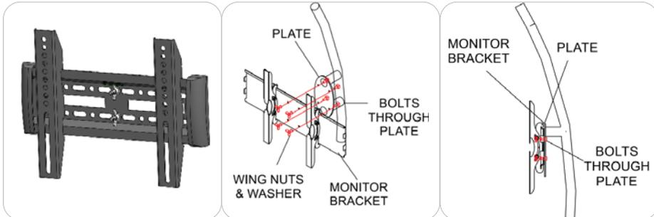
Remove the fastening hardware from the monitor mount bracket. Protrude the bolts through the tube frame plate. Fasten the monitor back plate onto the tube frame securing it with the provided wing nuts and washers.
