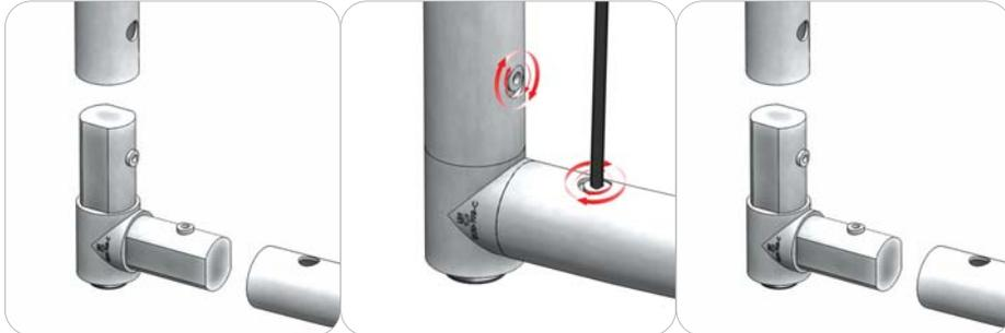
Compress one unlocked end of the connector and slide it through one tube end. Compress the other end of the connector and slide the second tube on. Lock both screws carefully using your allen key tool. Be sure to lock securely, but do not over tighten.
