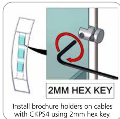
Install brochure holders on cables with CKPS4 using 2mm hex key.
