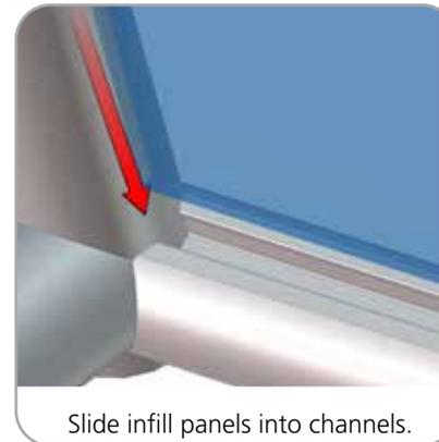
Slide infill panels into channels.
