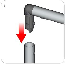
Fourth, take the male end of the plastic connector and snap it into the spreader tube open end.
