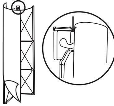
Use hook on panel and magnetic strip to secure graphic. 7
