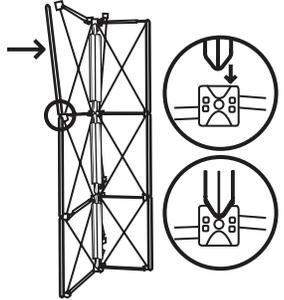
Continue placing channel bars around frame; slide into triangular groove to secure. 6
