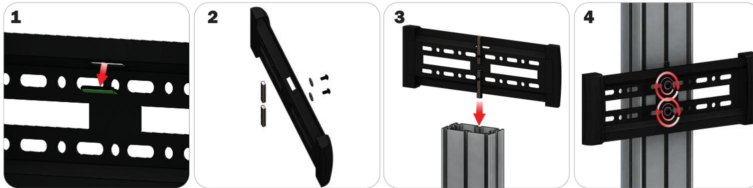
Locate all components needed to assemble the monitor mount with the channel connection B method. You will need (1) monitor bracket, (2) LN-LCD-SCW, (2) LN-100, and (2) washers.
